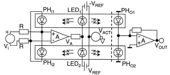
Fig. 1. The very simplified schematic diagram of the analog optical coupler realized.
