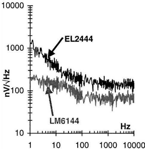
Fig. 3. Noise of the optocoupler when the photodiodes are operated at  $100 \text{ nA}$ , the noise floor is dominated by the Operational Amplifiers used, EL2444 (upper line) and LM6144 (lower line).
