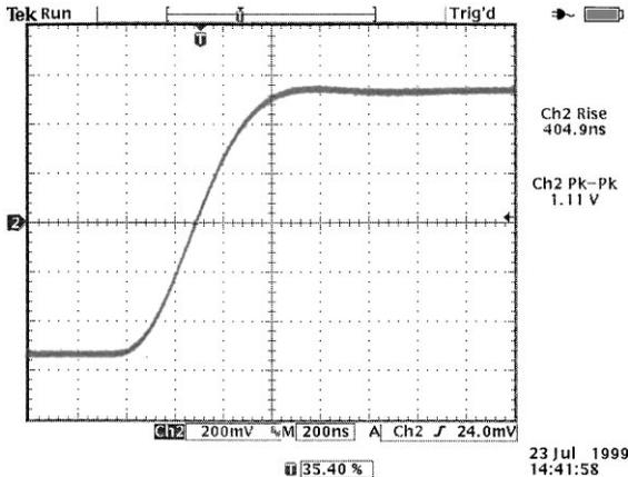
Fig. 2. A Tek photograph of the step response of the optocoupler. The horizontal scale is  $0.2 \mu\text{s}/\text{div}$ , the vertical scale is  $0.2 \text{ V}/\text{div}$ .
